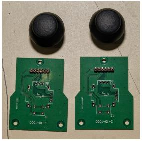
Like the low-profile receptacles, these are both J1 in the schematic. These may be a tight fit into the solder pads, be careful to not crush any of the leads.
