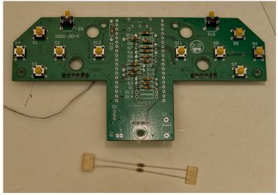
These are R13 and R14 in the schematic. These resistors limit the current to each colour of the Bi-colour LED, preventing the LED from drawing too much current and damaging itself.
