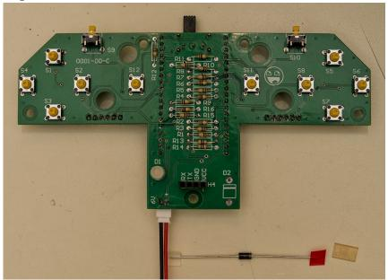
This is D2 in the schematic. Like the keyed power connector, this diode helps prevent reversevoltage events, though it takes a more active approach: acting like a one-way valve which won't allow power to flow if it is connected backwards.
