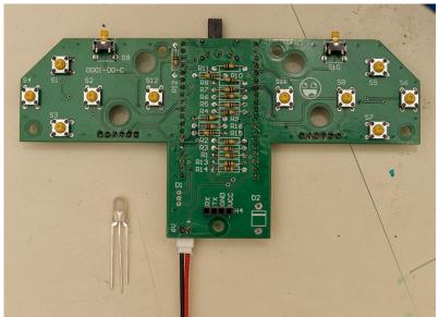
This is D1 in the schematic. This LED has 2 colors (Red and Blue) with a common cathode (ground) lead.
