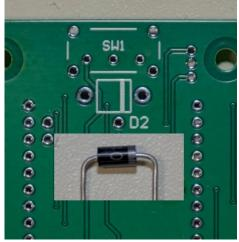
*Tip: Like the resistors, you can bend the leads of the diode once it's placed on the PCB to help hold it in place while soldering.*
