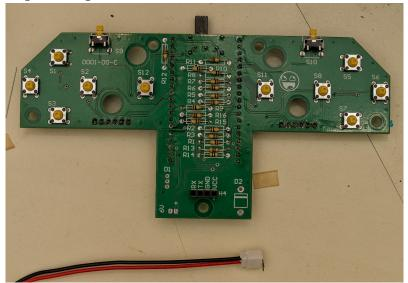
This is K1 in the schematic. This connector is keyed so you cannot plug it in backwards, helping to prevent reverse-polarity voltage events which could damage the controller.
