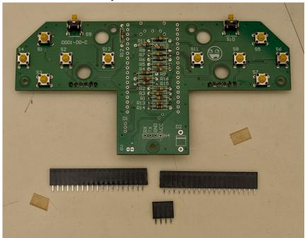
These are U1 and H4 in the schematic. U1 is actually the ESP32 module, but it is placed into these 19 pin headers rather than being soldered directly to the board. **The 4 pin receptacle goes on the top face of the board (the side with the buttons) and the 19 pin receptacles go on the bottom face of the board.**
