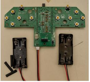
These holders do not have a schematic symbol, as they connect via the keyed JST power connector instead. The 3 pieces of heatshrink tubing are also used in this step to cover some wire-to-wire solder connections.
