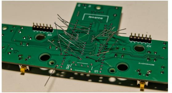
7. Solder the 470 ohm resistors to the main-board PCB
