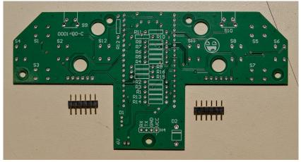
These headers are H2 and H3 in the schematic for the right and left joystick module respectively.
