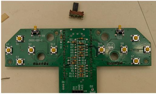
This is SW1 in the schematic. This switch goes on the bottom of the PCB.
