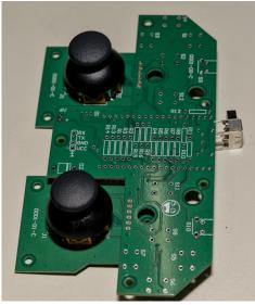
4. Solder the 6mm vertical buttons to the main-board PCB
