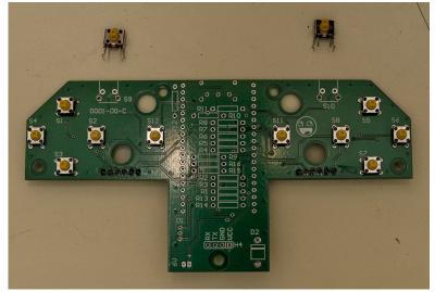
These are S10 and S11 in the schematic. Due to the previous step, these should need no special support when soldering, and they also some slight locking like the vertical buttons.
