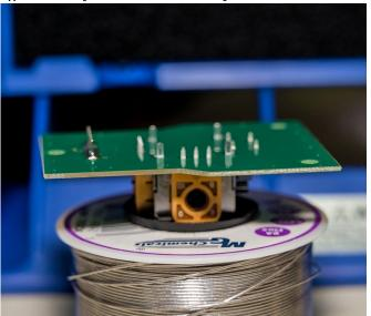
3. Solder the low-profile male headers to the advanced main-board PCB
