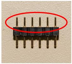
*Tip: attaching the joystick module PCBs to these headers and using the switch's pins to prop up the board can help keep it stable while soldering these headers.*
