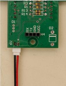
Tip: by bending the wire harness that is plugged into this connector can help hold it stable while soldering. After soldering the connector, you can disconnect the wire harness if it is in the way.
