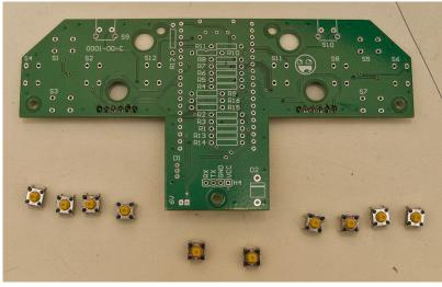
These are labelled S1-S8, S11, and S12 in the schematic.
