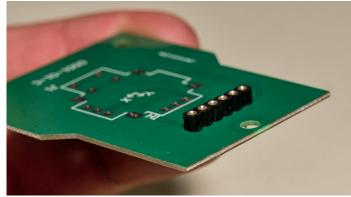
Tip: Using the other headers/receptacles on their sides placed on the opposite side of the board by the part number, you can keep the board level while soldering (the above was placed onto the below image for soldering, making a "receptacle sandwich")
