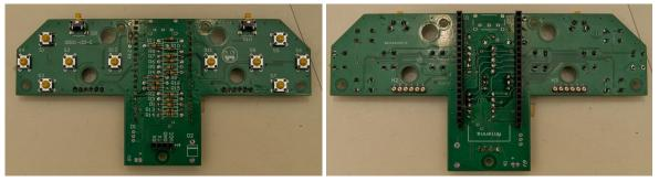
9. Solder the main power switch to the main-board PCB
