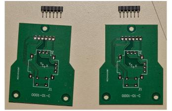
These are both H1 in the schematic, as both joystick module PCBs use the same page in the schematics. The holes for these headers is also larger than typical for these headers, this is to reduce the overall height of the controller slightly. The black plastic of the receptacle should sit flat on the PCB face like the image below.
